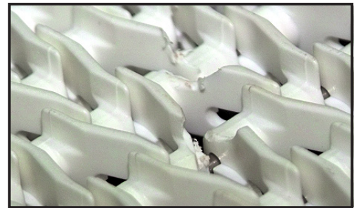
Inspect Chain for broken links
