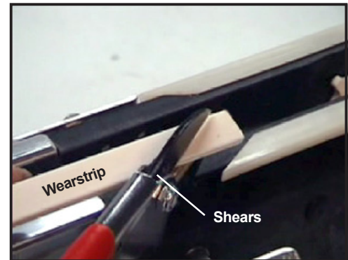
Figure 13: Cut wearstrip at 60° angle
