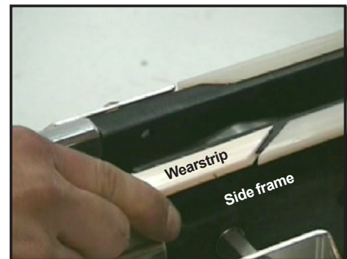
Figure 14: Slide wearstrip into side frame
