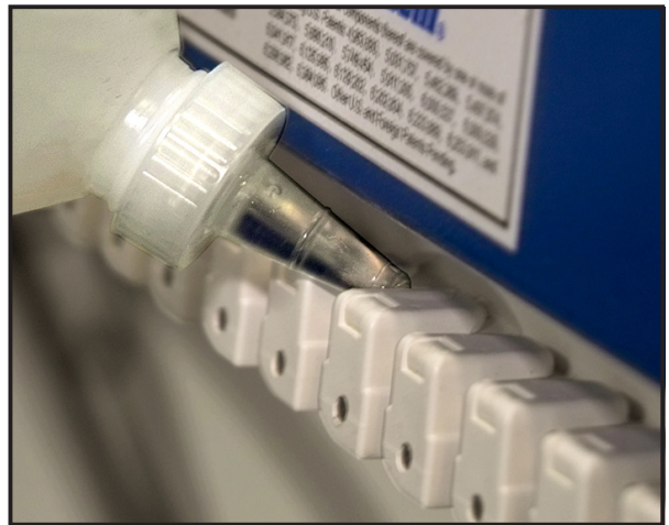
Lubricate the conveyor wearstrip with silicone oil
