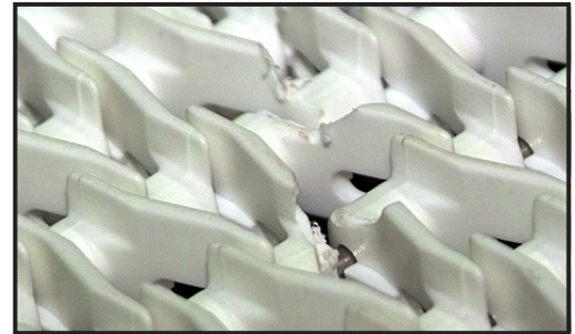
Inspect Chain for broken links
